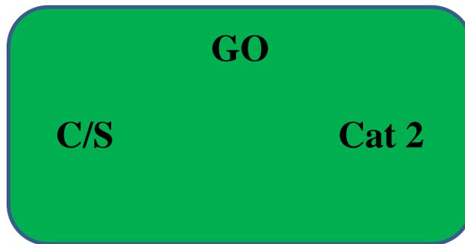
Figure 4: Green light pad showing permission to access (GO) also showing the Confined space category as Cat 2
